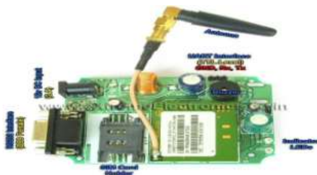
Fig.7 (b): Developed GSM Module
